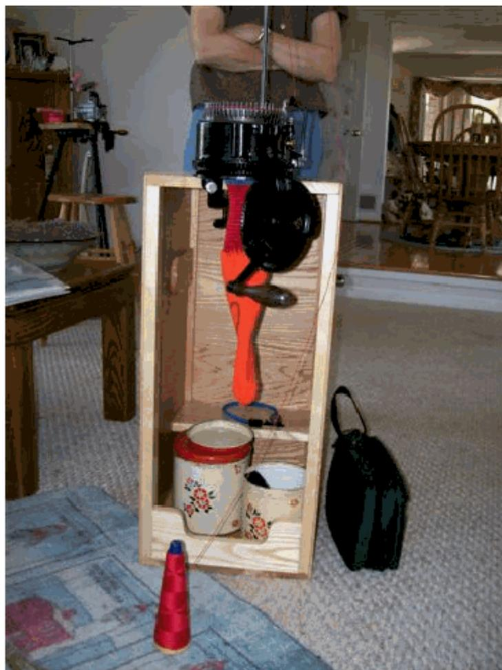
One of the problems beginners have with sock machines is setting up the yarn supply to guarantee zero back tension. It looks as though one could simply feed the yarn from a skein, ball, or cone directly into the machine. Sooner or later, the yarn will snag, and that happens when the heel is being turned and the last needle to knit is at a critical position.
