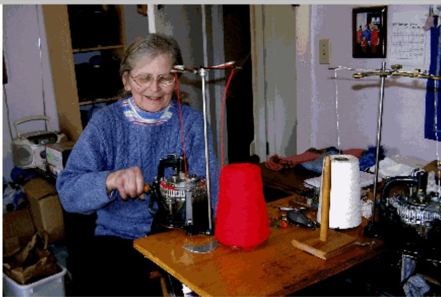
In an e-mail to Elsie, I asked how she manages some of the problems encountered when using the ribber and separating the sock from scrap material. A specific problem is holding the yarn down on the needles at the location where the ribber lug pinches yarn against the lug or post inside the cylinder.
